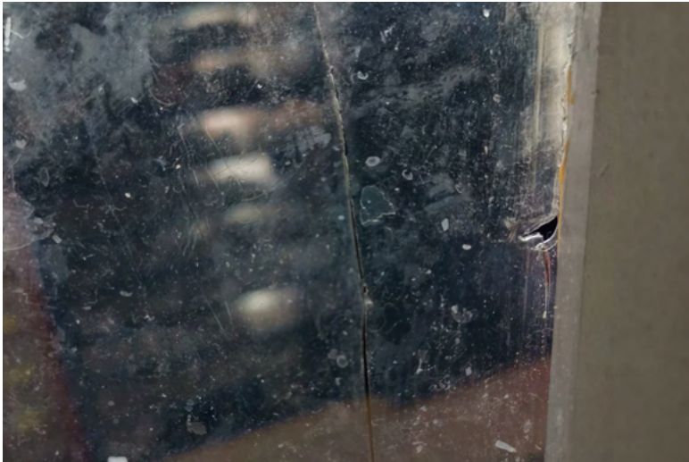
An extreme case of FEP film damage
